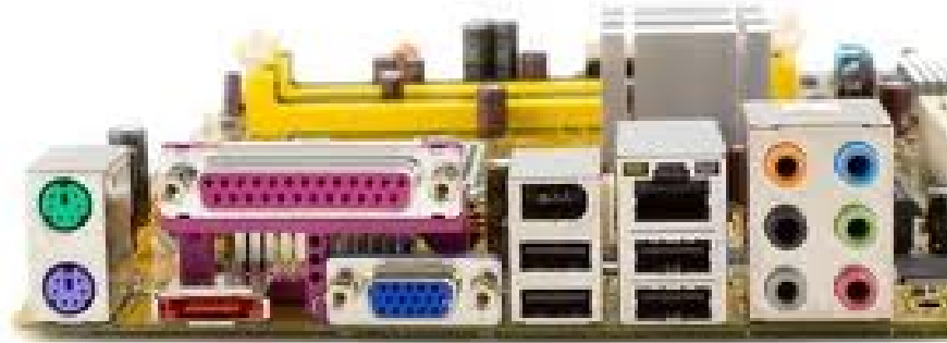
Figure 12 Typical Shielded I/O Connectors mounted directly on PCB
