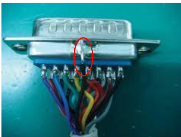
Figure 28 Left – Pigtail termination,
